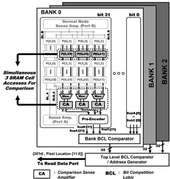
Figure 5. Overall Architecture of the VIP memory
