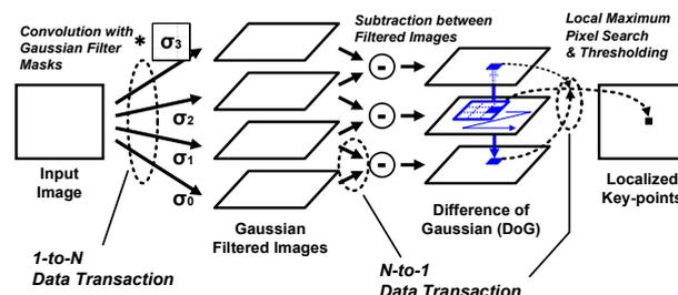
Figure 1. Overall Flow of the SIFT Computation
