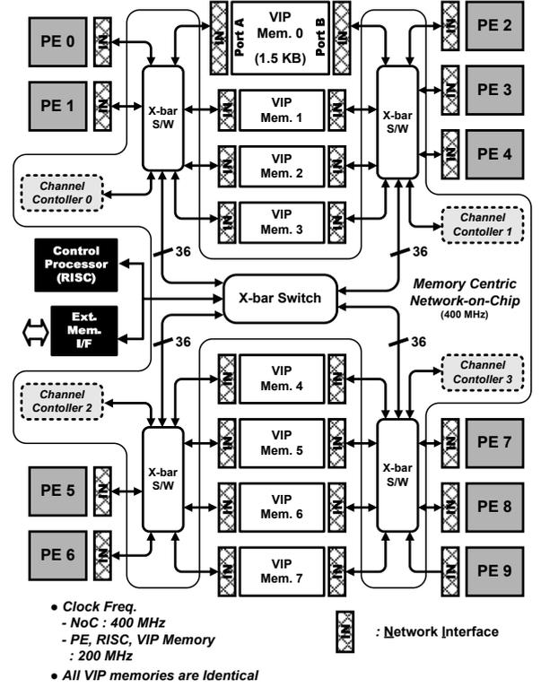
Figure 2. Architecture of the Proposed Object Recognition Processor based on the MC-NoC
