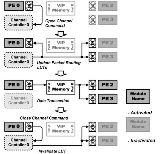
Figure 3. Operation of the MC-NoC
