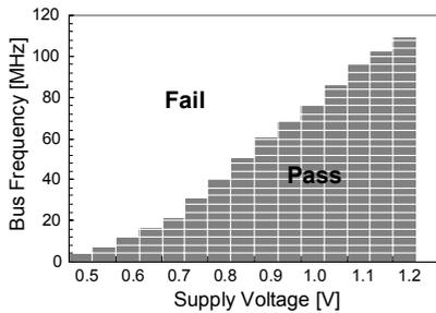
Figure 8. Frequency versus supply voltage plot at body temp.
