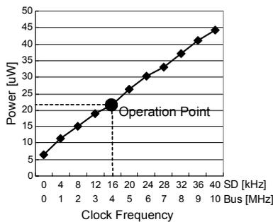
Figure 9. Power Consumption by Clock Frequency with 0.6V VDD
