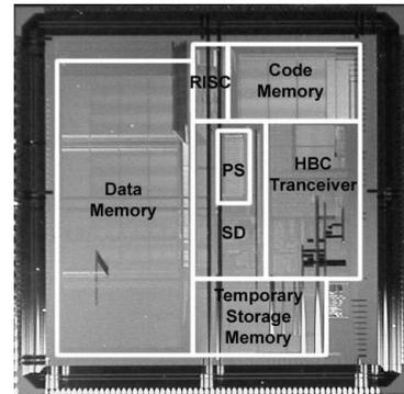
Figure 7. Photograph of the BSN processor
