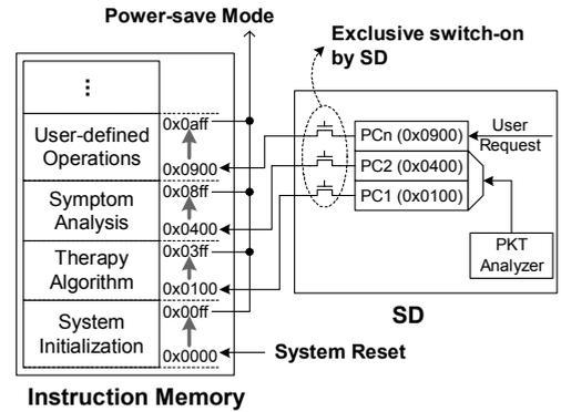
Figure 6. PC Transition with IPEEP Scheme
