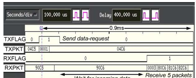
(b) Measured Packet Transaction by SD Operation
