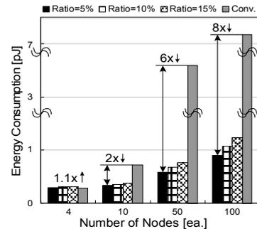
Figure 4. Energy Consumption for Scheduling Nodes
