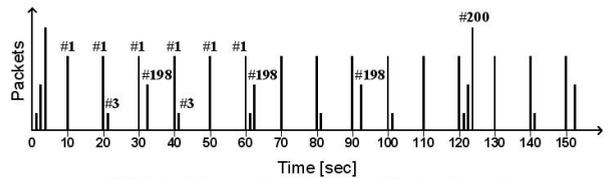
(a) Packet Transactions measured for 4 nodes with 10s(#1), 20s(#3), 30s(#198) and 120s(#200) periods
