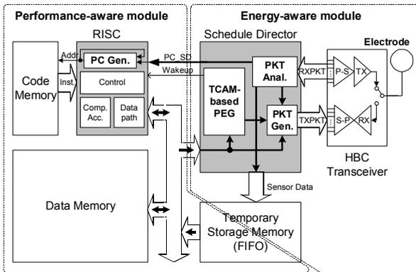
Figure 2. BSN Controller Architecture for Dual-mode Operations
