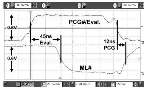
Fig. 7. Measured Waveform of PS operation with 0.6V VDD
