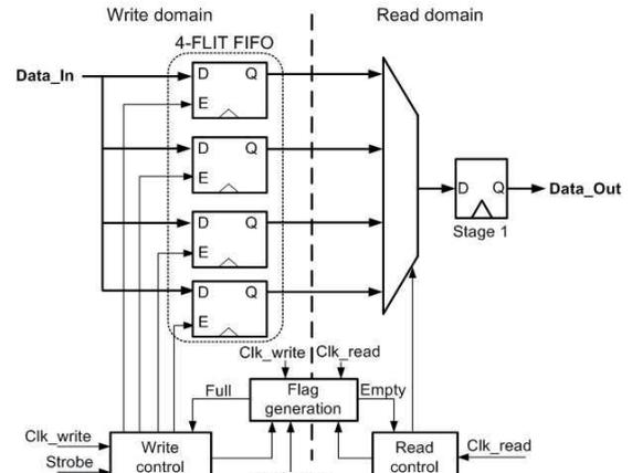
Figure 6. FIFO-based synchronizer
