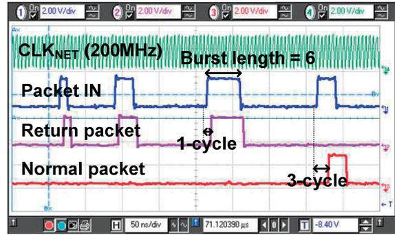
Figure 9. Measured waveforms of the NoC packet signals
