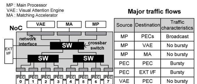
Figure 1. Object recognition processor with major traffic flows
