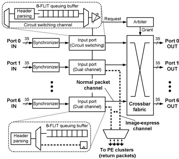
Figure 4. Block diagram of the proposed crossbar switch
