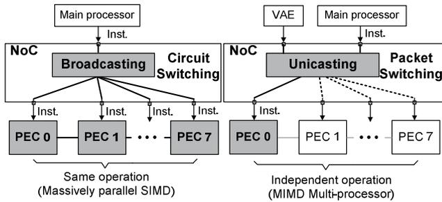
Figure 2. Dual-mode configuration
