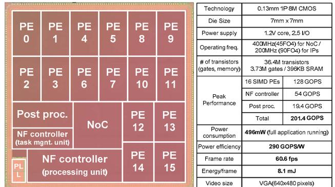
Fig. 5 Chip micrograph and feature summary
