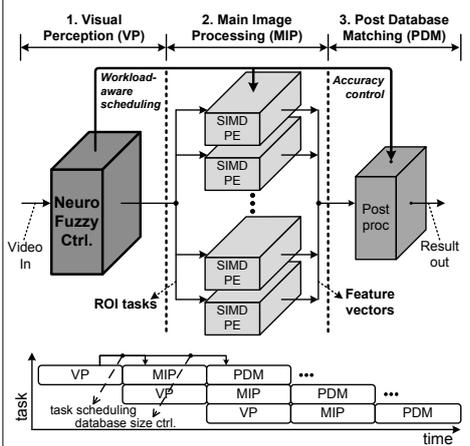
Fig. 1 Proposed neuro-fuzzy controlled multi-core architecture
