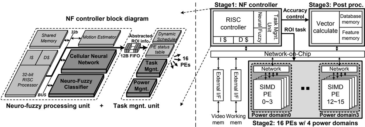
Fig. 3 Block diagram of the proposed NF controller and overall processor
