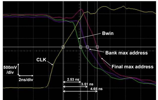
Fig. 8. Measured Waveforms of VIP-RAM
