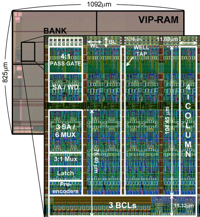
Fig. 7. Photograph of the Fabricated Chip and Core Layout
